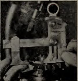
Check Side Clearance of 4 x 3/4 Inch, Alternate Tooth Mill
